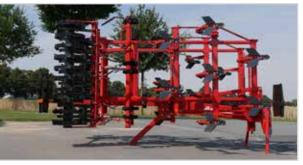
Either mounted rigid or fold – both version are very compact for a good centre of gravity and reduced lifting capacity. For safty parking extra legs are available.
