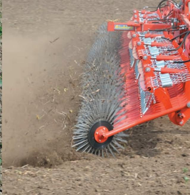
**6.5 mm / 0.26" thick spring steel tines**, cast into an inclined plastic disc do the job. Each of these 50 cm / 9.7" big star wheels is suspended separately, therefore they adapt perfectly to any surface irregularities.
