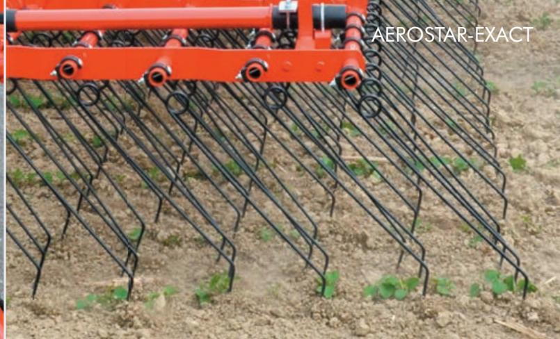
The tine with a diameter of 7 mm / 0.28" and a length of 600 mm / 23.6" offers many advantages in **special crops**. And it also adapts very well to **uneven soil conditions**.
