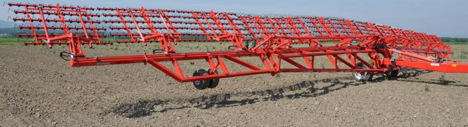
All sections of the semi pull type version of the AEROSTAR are attached to suspend beams. These beams are hydraulically controlled (hydraulic level adjustment).
