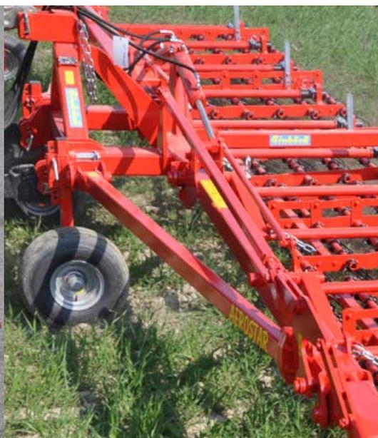
Larger working widths, especially with shear retraction, are made possible through a large **angular support brace** that will keep the frame from swinging even at higher speeds and aggressive tine position.
