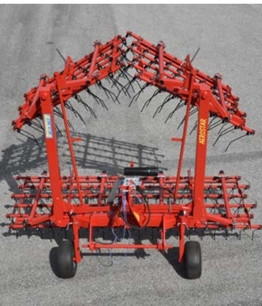
Folding the side sections will reduce the width of the AEROSTAR to a **transport width of only 2.6 m to 3 m / 8.5 ft to 9.8 ft.**
