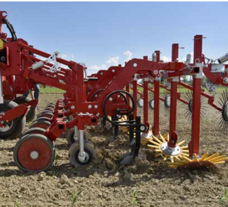
Parallelogram with 2 Farmflex-wheels
