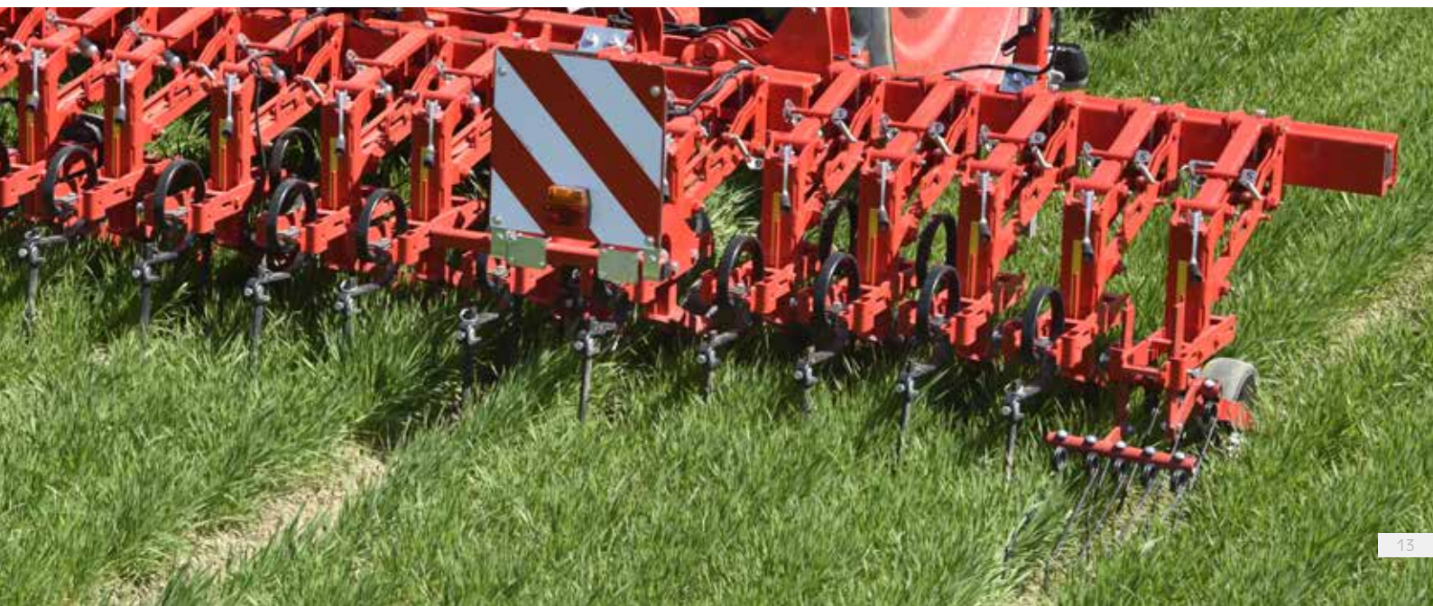
Hinged crop protection shield for hoe section CHOPSTAR 1-30 / 11.8" from a row spacing of 25 cm / 9.8" (optional)
