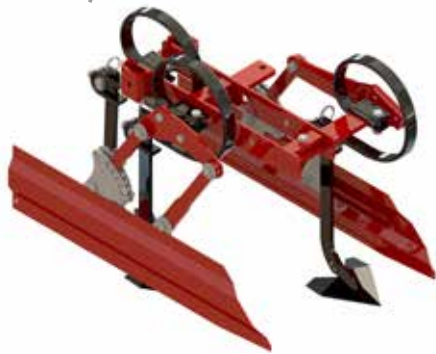
Hoe section CHOPSTAR 3-60 / 23.6", with hinged crop protection shields and vibrotines for shallow operation
