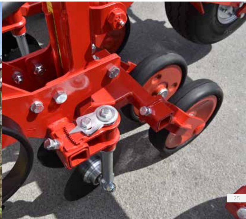
Hoe element with angle knife and vertical cutting disc
