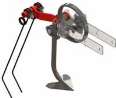
Adjustable weeder tines for CHOPSTAR 1-30 / 11.8", CHOPSTAR 3-60 / 23.6" and CHOPSTAR 5-90 / 35.4". The outer tines on each section can be turned around, in order to push soil away from or towards the row (not on CHOPSTAR 1-30 / 11.8").
