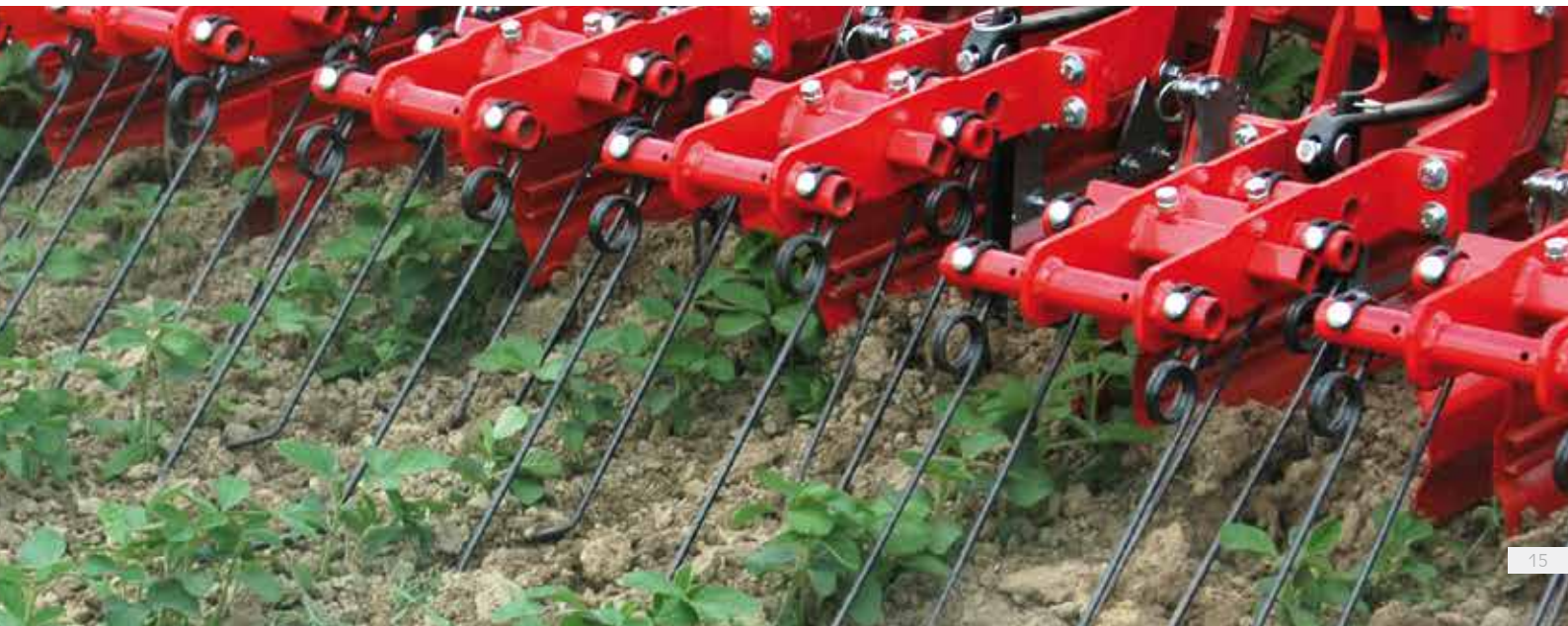
Hoe section CHOPSTAR 3-60 / 23.6", with hinged crop protection shields and vibrotines for shallow operation
