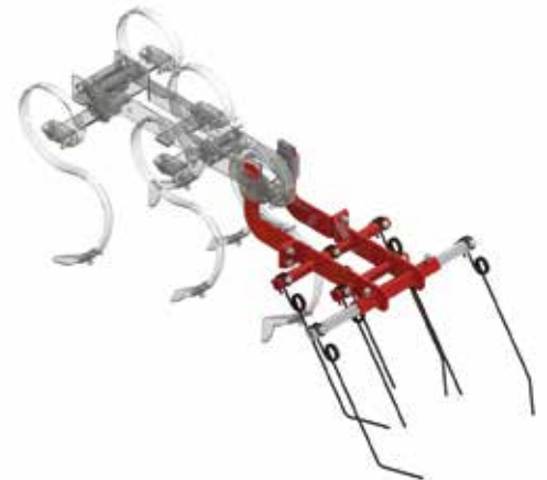
Adjustable weeder tines for CHOPSTAR 1-30 / 11.8", CHOPSTAR 3-60 / 23.6" and CHOPSTAR 5-90 / 35.4". The outer tines on each section can be turned around, in order to push soil away from or towards the row (not on CHOPSTAR 1-30 / 11.8").
