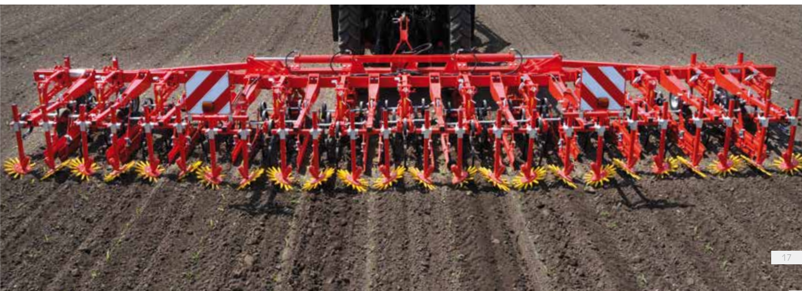
For crops that require shallow hoeing, the hoe section CHOPSTAR 5-90 / 35.4" is also available with shallow working vibrotines (optional)
