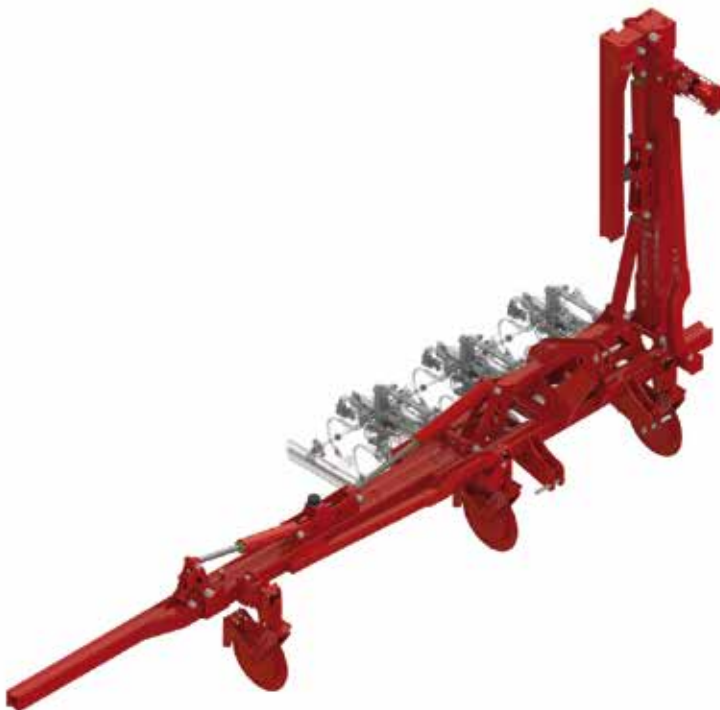
Frame for a rear-mounted machine with double folding frame (4 hinge points) for reduced transport width for large machines
