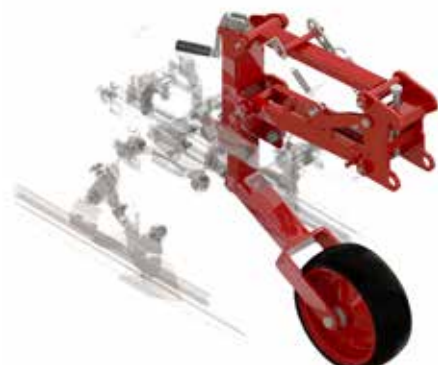
Hoe element parallelogram on rear-mounted machines
